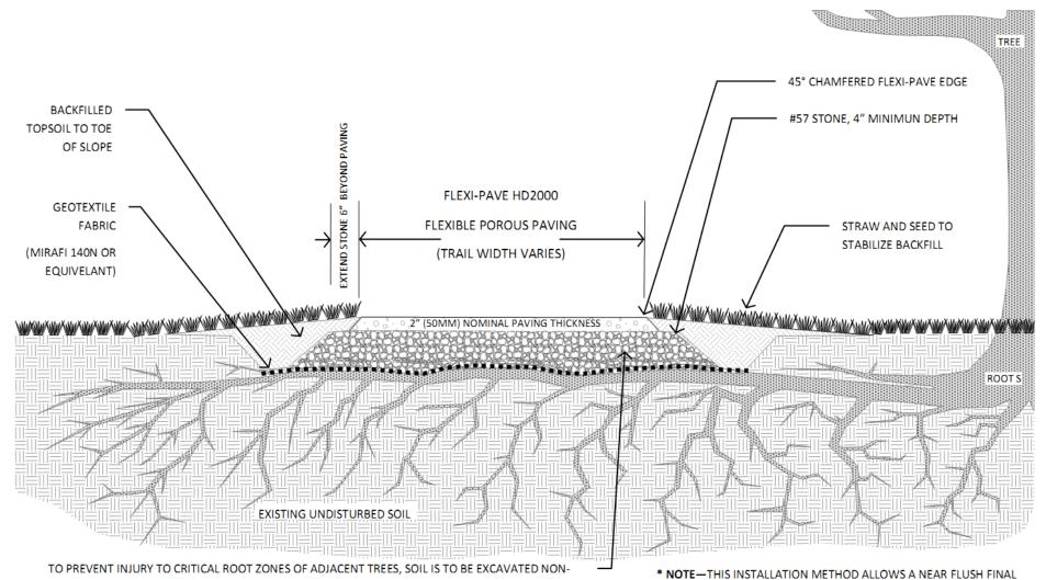
TO PREVENT INJURY TO CRITICAL ROOT ZONES OF ADJACENT TREES, SOIL IS TO BE EXCAVATED NON-INVASIVELY TO ROOT DENIAL DEPTH USING SUPERSONIC AIR KNIFE. THEN FABRIC AND STONE ARE TO BE INSTALLED OVER AND AROUND ROOTS. ROOT PRUNING MAY BE PERFORMED BY ARBORIST AS NEEDED ON SELECTED ROOTS <2" IN DIAMETER PROVIDED NO MORE THATN 15% OF CRITICAL ROOT ZONE IS REMOVED.
