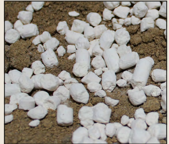
FIGURE 1: ORC-A PELLETS ARE APPROXIMATELY 3-10 MM SIZE
