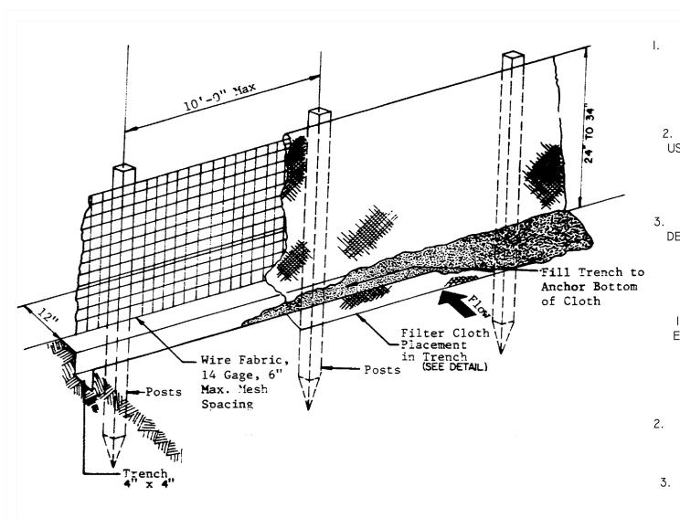
WHEN WIRE SUPPORT IS USED, STANDARD STRENGTH FILTER CLOTH MAY BE USED AND POSTS SHALL BE SPACED 10 FEET ON CENTER MAXIMUM.
